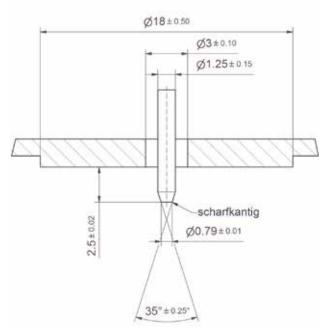
As for standardized measurements minimum sizes are required, this can often cause a limitation. For conventional units, a specimen with a minimum wall thickness of 6 mm and a 18 mm supporting space in diameter is presupposed.
