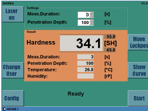
The display remains until the next keystroke or measurement is made. Displayed are single measurement values in Shore An, besides values of temperature and device settings. If the data results are within defined limits the basic colour is green, if they are outside the min-max control the colour is orange and it is red for incorrect measurements.
