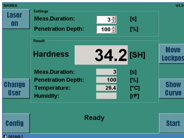
The measurement procedure is fully automatic. If the device is exposed to stronger vibrations, the accurate determination of the surface location needs more time and the measurement process is prolonged, respectively this can cause increased measurements deviations.
